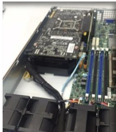
Ultra compact: 1 active-cooled Dual- Slot GTX-GPU in 1U...
