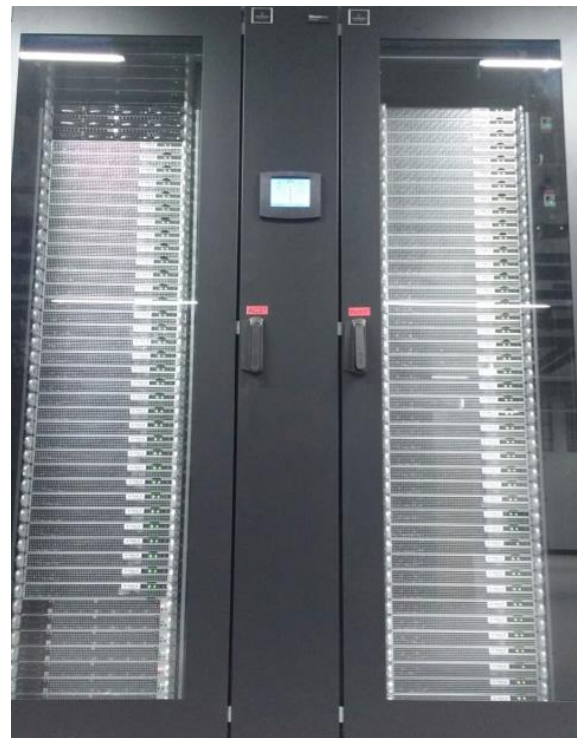
Rack 1 + 2 each have 42x MUSTANG® systems systems/ SuperMicro BTO 1U Super Server incl. 1x E5- 2630v4+NVIDIA GTX 1070/GTX 1080...
