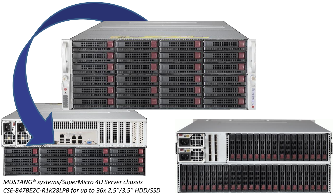
MUSTANG® systems/SuperMicro 4U JBOD-Chassis SC417E16-R1K28JBOD for up to 72x 2,5" HDD/SSD
