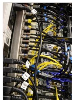
Rear side with 1GB as well 56GB/s network and DCLC leads ...
